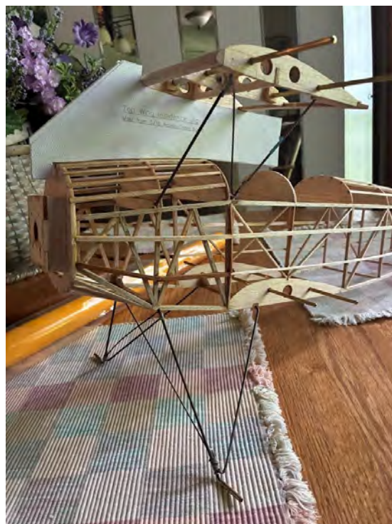
Above: Bob Curry sets the top wing's incidence with a jig between the wing and fuselage.
