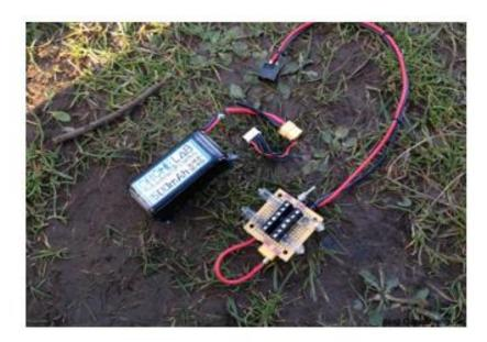
Don't forget to save the XT60 and balance connectors for future use! If you have damages on a good pack you can use them for replacement.
