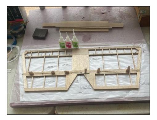
Here you can see the horizontal stabilizer & elevator is completely assembled, glued and pinned.
