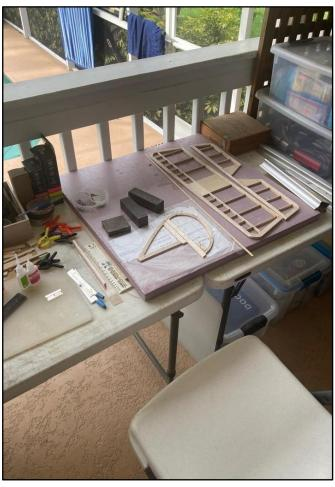
The second image (above right) is showing the progression on the horizontal and vertical tail assemblies. As you can see in both images, the plans or "template" are laid out on a flat, smooth surface and covered with wax paper to allow the template to show through. This allows the parts to be assembled easily while protecting the originals just in case he wants to build another one down the road.
