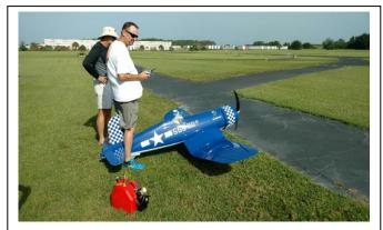
Here are a few more pictures of Mike Zellars new F4U-1D 1:4.5 scale Corsair by CARF Models. As previously mentioned, the plane has a 110" wingspan, is powered by a Moki 250cc radial engine with electric start (bottom left), Sierra retracts, full functioning flaps and a Solo adjustable prop. Only 10 servos are required to operate the control surfaces and all of the little extras....
